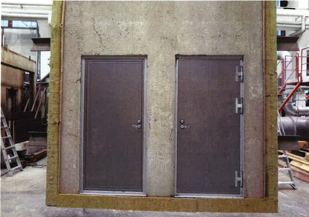
Figure 1. Exposed side of the test specimen prior to the fire test.
