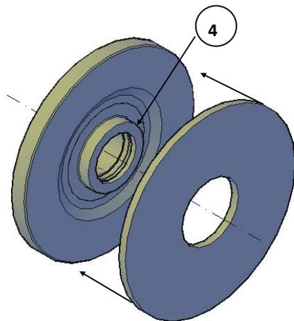
Fig. 8. Gear side of the clutch and the friction lining
